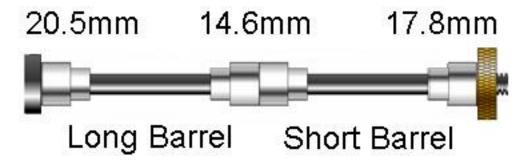
Turn outside diameter of the pen blank down to dimensions above.
